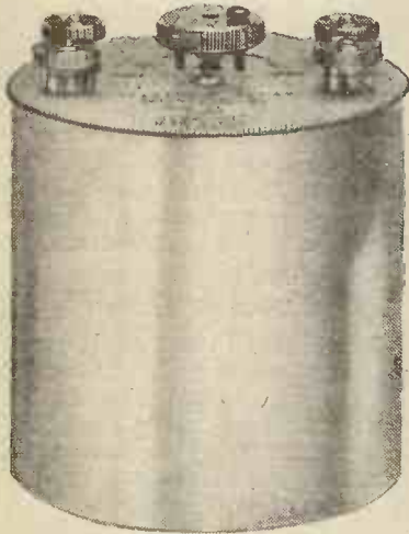
An early type of Brown Relay, used for amplifying signals.
