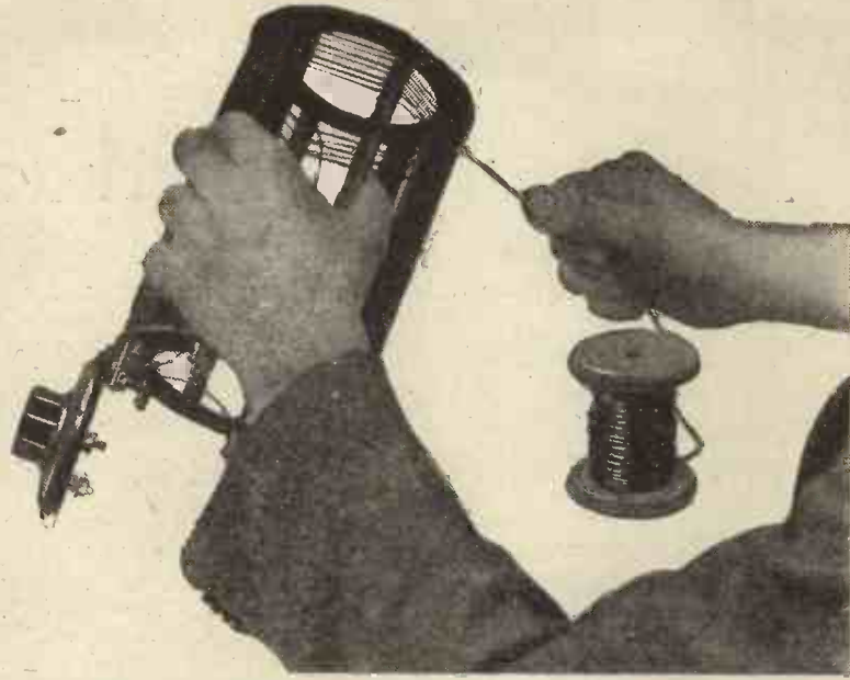
Showing how the coil is wound. Although the wire must be tightly wound, a stiffening ring supplied with the former removes the risk of crushing the side strips inwards.
